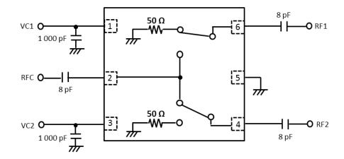
The application circuits and their parameters are for reference only and are not intended for use in actual design-ins. This device is used it is necessary to use DC Block Capacitance.
